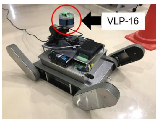
Fig. 6 Exploration robot equipped with VLP-16
